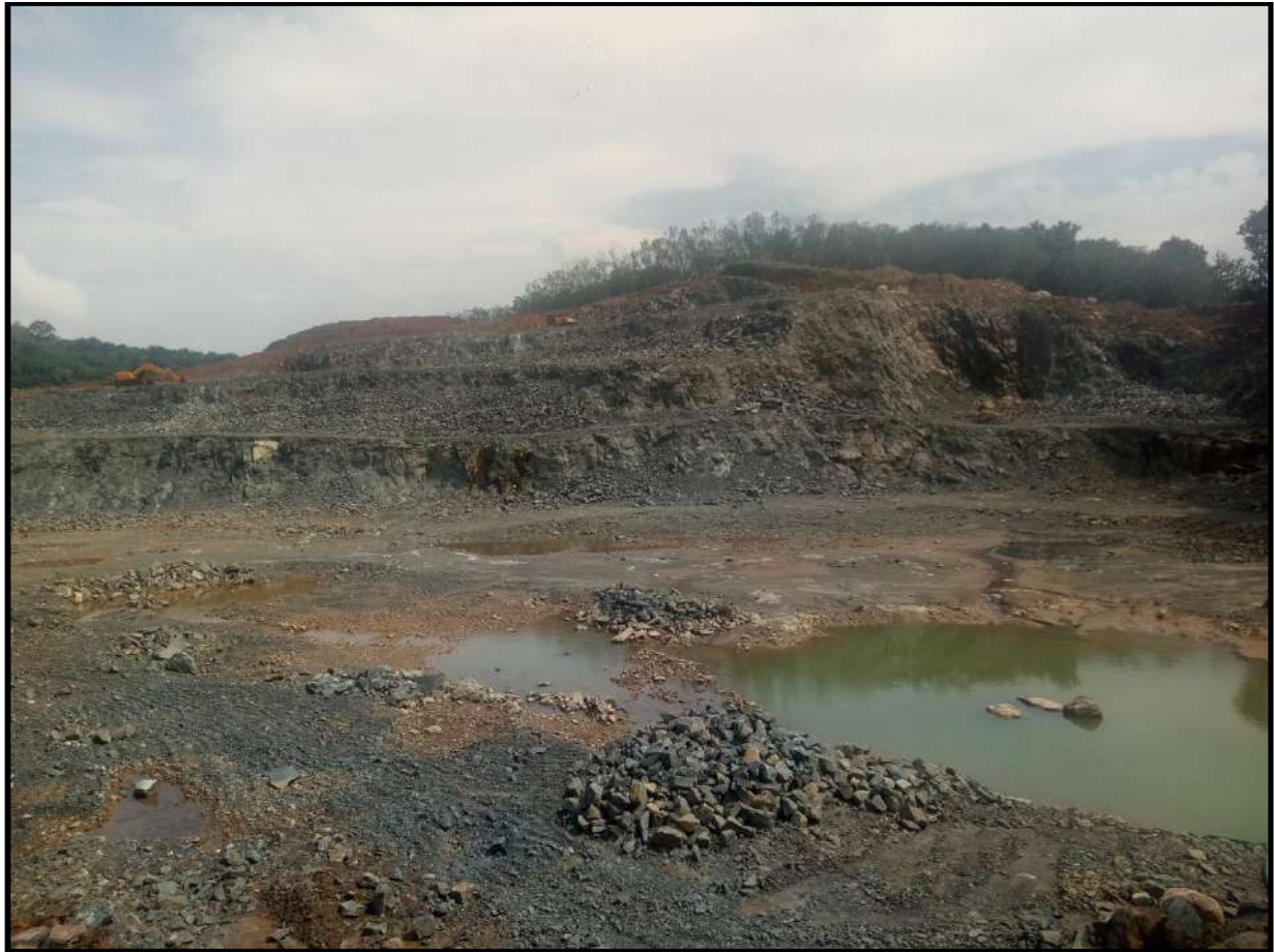
The photograph showing bench type mining
